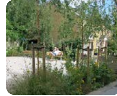
Waltham Village Square | Rain Gardens Full of native shrubs and flowers planted in a depression to temporarily hold and soak-in rain water runoff from roofs & driveways
